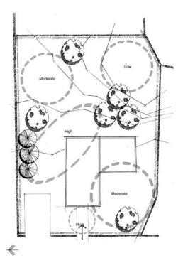
Fig. 1.3: A site plan showing water-use zones.
