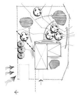
Fig. 1.2: A site plan showing site characteristics (views, drainage, ... etc).
