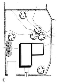
Fig. 1.1: A site plan showing the location of structures and existing features.
