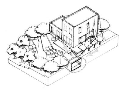
Fig. 3.8: An active rainwater harvesting system.
