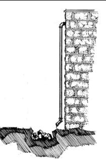
Fig. 3.6: Rocks may be used to disperse water coming out of a downspout.
