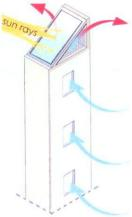
Passive Cross ventilation in each apartment is created by opening high windows on top of main entrance door of each apartment to create air flow through the vertical structure of the stair case acting here as a wind tower too.
